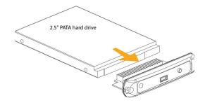
**4** Slide the drive tray, with drive attached, into the enclosure.
